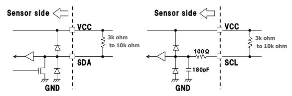
Note: The SCL terminal is connected to GND with a 180 pF capacitor. Please check that there are no problems with data transmission before use.
