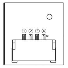
Figure 2 Pin Configuration (Top View)
