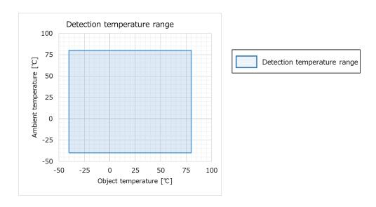
Figure 4 Detectable temperature range (for reference)
